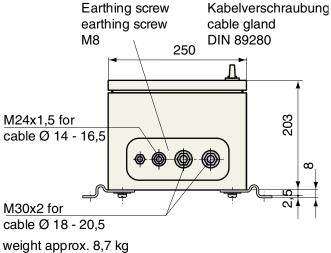
cable gland according to DIN 89280 for MGCG cable
