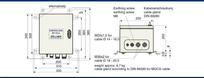
Standard control box (supply voltage 380 / 440 V - control voltage 115 / 220 V) - other voltages on request
